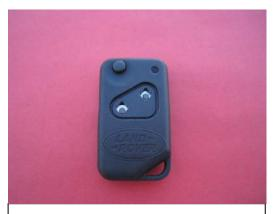
Your remote control should look like the one above, ready for fitting new Silicone pad. DO NOT USE any lubricants or detergents for cleaning grooves as it will affect firm seating of a pad.
