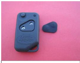
Press fit new pad in, making sure it sits firm and flat in groove all around
